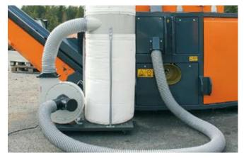
**THE SAWDUST EXTRACTOR** traps all sawdust neatly into a container. A compact model runs on mains electricity, the larger exhauster on 3-phase power.
