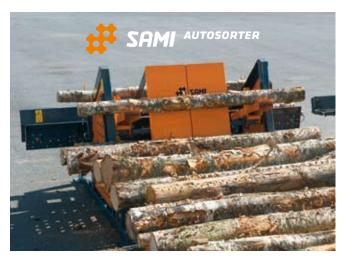
**AT WIDEST, SAMI AUTOSORTER** consists of a loading table, a sorter and a transfer conveyor. SAMI Autosorter integrated in SAMI Autochopper – the entire log splitting process is automatic.
