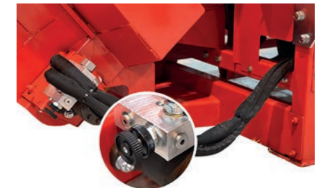
Outfeed conveyor speed control valve as easy-to-install accessory.
