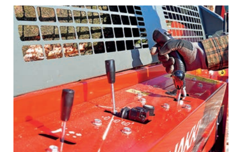
Easy-to-use control panel where infeed, cutting and splitting are all controlled with just one joystick.
