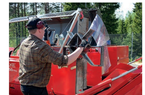
Replacing the splitting blade is fast and safe thanks to the detachable winch.
